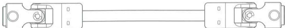
BC33 ×1 18085926 プロペラジョイント L Propeller joint (long) Antriebs-Gelenkwelle (lang) Cardan central article (long)
