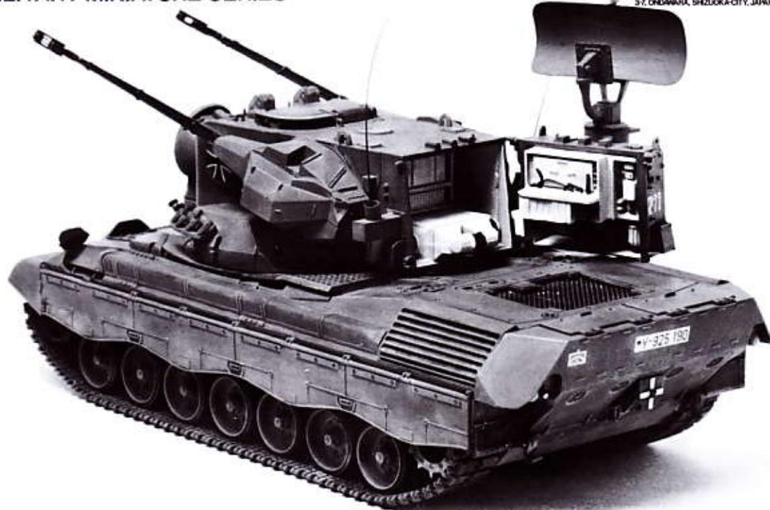
Basis of the Gepard weapon system is the remarkable Oerlikon-Contraves 35mm which was developed and put into production in the early 1960s. To combat modern jet aircraft approaching on the battlefield at tactical attack heights, a very high rate of fire was needed coupled with a high muzzle velocity. The 35mm calibre was found to be the optimum size for the best combination of weapon weight and effectiveness.
